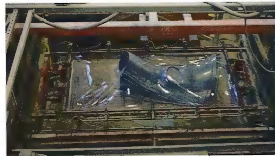
Heat forming of 1/8" polymer resin over the grey protective layer
