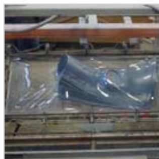
The design team thermoformed the panels at Warner Bros. Staff Shop. (Courtesy B+U)
